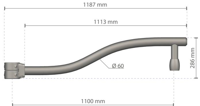
The drawings show the pole arm with Ø 89 pole collars, suitable for Steel Black poles fixing. The pole arm is equipped with Ø 79 pole collars for Steel Red or Steel Green poles fixing. (Ø 79 pole collars are shown in the pictures at the bottom.)
