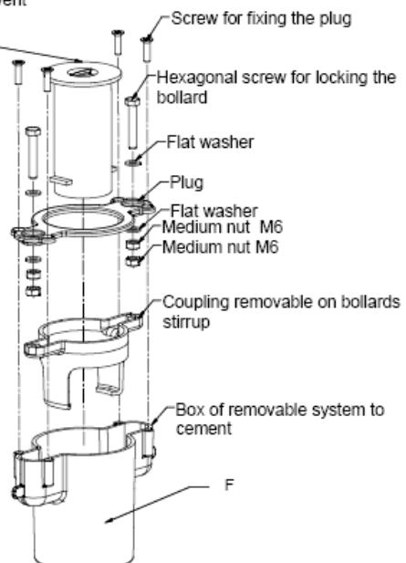
To remove this item, follow the instructions in reverse order. This system is equipped with a plug to be used after removing the bollard.
